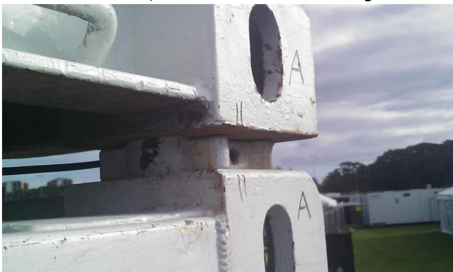
Notable among the changes is the inclusion of fully automatic twistlocks and automatic container locks (the latter have no twisting element, nor any moving parts).
