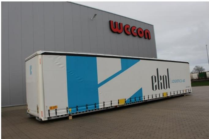
Internal measurements are 14.83m x 2.48m x 2.97m.
