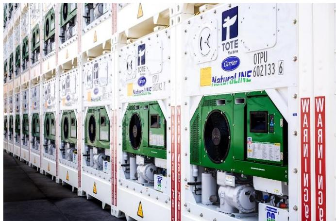
NaturaLINE units use CO<sub>2</sub> refrigerant, also known as R-744, which has an ultra-low GWP of 1, in comparison to GWPs that range from 600 to nearly 4,000 for refrigerants used in other container systems.
