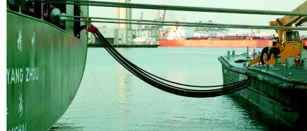
Electricity from the grid will most likely be used more and more to charge batteries for ship operations in ports, but also for propulsion of relatively small vessels.
