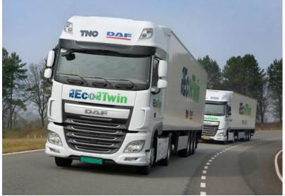
consortium, formed by NXP, DAF, TNO and Ricardo "Roadlink" uses the wireless communications standard IEEE 802.11p combined with NXP radar technology so the trucks within the platoon securely exchange information in real time and automatically brake and accelerate in response to the lead truck.
