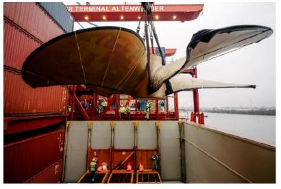
waiting: a 92-ton propeller from Shanghai with a 9.20meter diameter.
