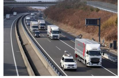
In the commercial vehicle sector, truck platooning will contribute to the reduction of fuel consumption and to lower CO2-emissions.
